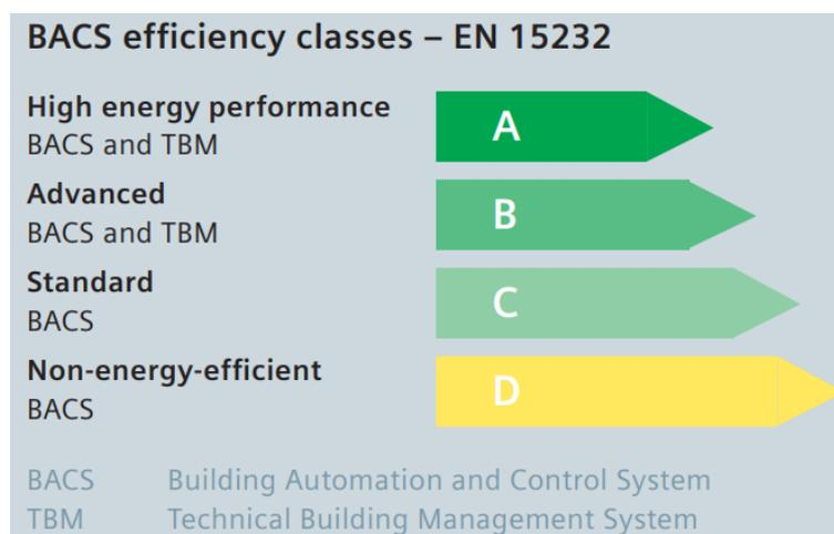
Figure 50: BACS efficiency classes – EN 15232 [20]
