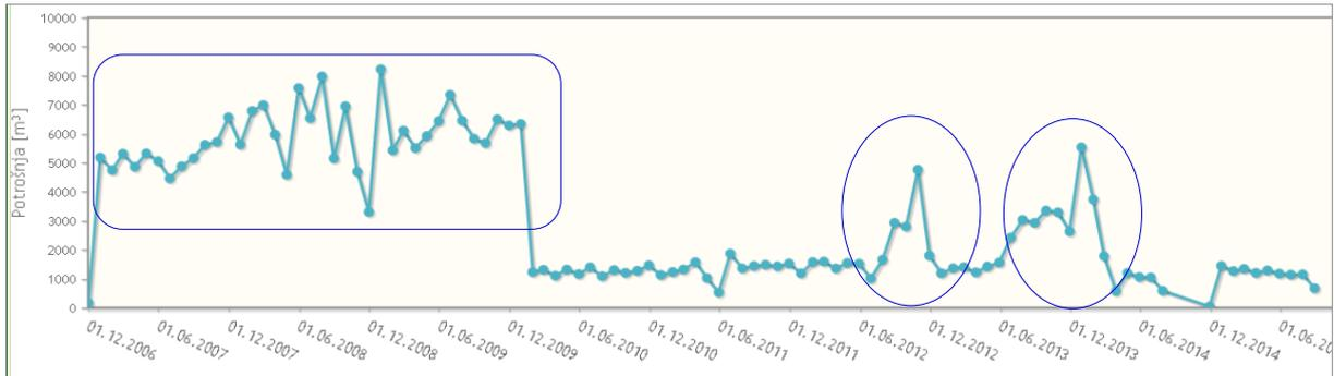
Figure 8: Increased water consumption due to cracked water pipes in the water distribution system outside a public building detected by EMIS
