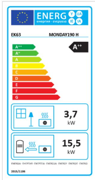
Figure 53: Energy label of a local space heater
