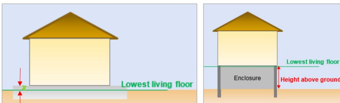
Figure 41: Base height – height above ground for non-elevated and elevated buildings
